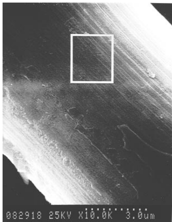
Figure 3. Scanning electron micrograph (SEM) of the surface of a C–SiO 2 coated carbon fiber.
